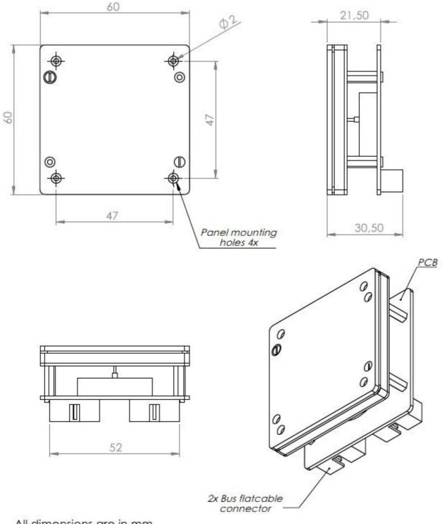
Flight Illusion Small Single Needle Assembly without Bezel
