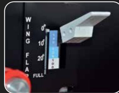
The flap lever moves in exactly the same way as in a real aircraft. The indicator shows the flap transition.
