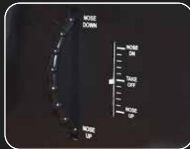
The panel features both an electrical and manual trim. The trim wheel moves while operated from the yoke and the indicator shows the position of the trim.
