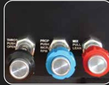
The Throttle-Prop-Mixture levers give you realistic control of your single engine aircraft ! The individual throttles are proportional.
